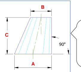
An oblique cone is a cone with its **axis not 90°** from its base. The top and base are parallel and true circles. It can be used as a reducer for offset pipes.
