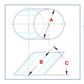
An oblique cylinder consists of the transition between two pipes of equal size whose center lines are offset from each other.
