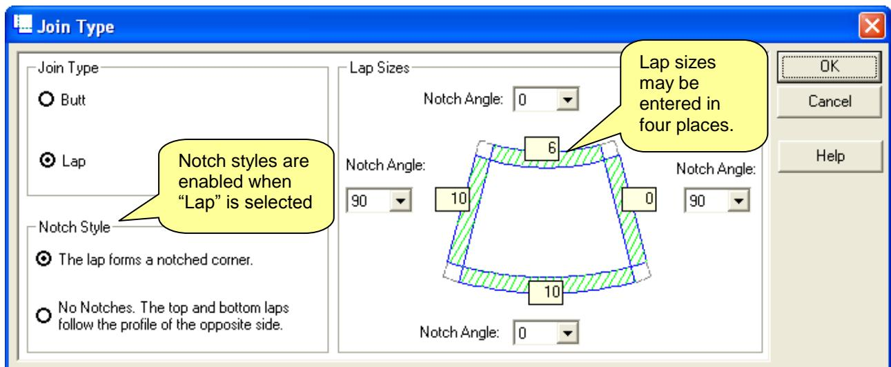
By default, the Notch Style “**Lap forms a notched corner**” is enabled. The diagram below shows the result of the settings applied in the dialog above. A lap of 10 is applied to the left end of the pattern, a lap of 6 is applied to the top edge and a lap of 10 is also applied to the lower edge.
