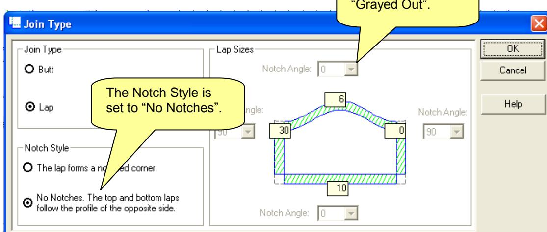
When the '**Notch Style**' option is set to '**No Notches**', no corner notch is formed and the profile is continued around the end laps. When this option is selected, the Notch Angle options are "grayed out" and ignored.
