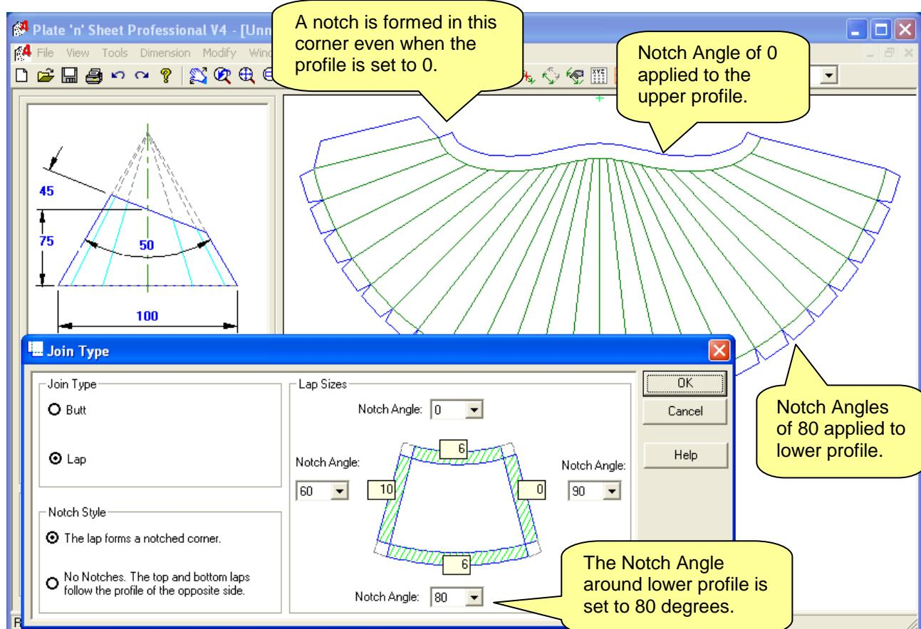
**NOTE:** A notch angle of 0 on the upper and lower edges means that no notches are applied around the profile, other than the notch in the “corner” formed between the end lap and the upper or lower profiles.
