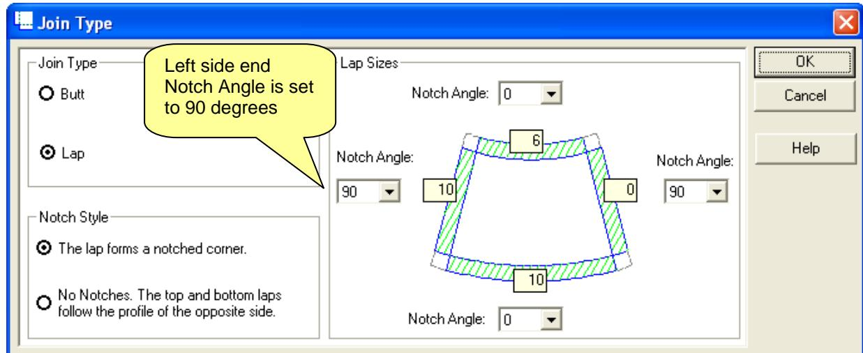
In the above example the Notch Angle of the left side end lap is set to 90. The notch angle is measured from the end line of the pattern. Changing the notch angle to 60 would give the following result:
