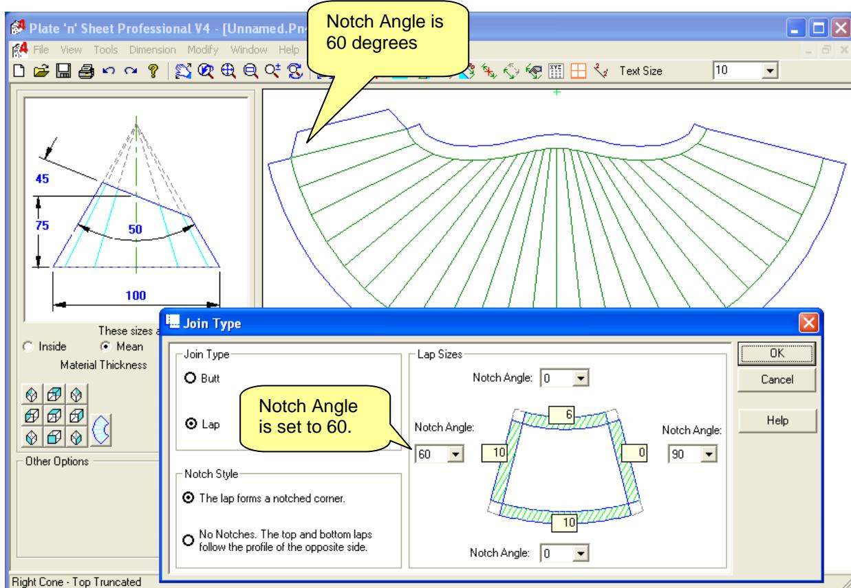
When a Notch Angle is applied to the **upper or lower lap**, notches are cut at each press line. The nominated notch angle from the last segment measured around the profile. The diagram below shows a notch angle of 80 degrees applied to the lower profile.
